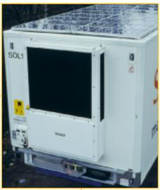
Sainsbury's is testing two solarpowered refrigerated trailers. The PV cells on the roof charge a battery, which powers the refrigeration system. Photo courtesy of DTI
