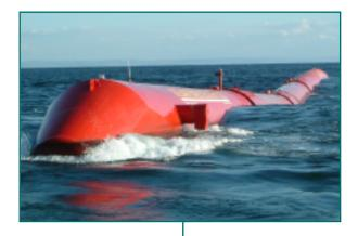
Pelamis near Orkney, Scotland Photo courtesy of Ocean Power Delivery Floating devices or barrages are generally found offshore. A good example is Pelamis, a wave-power project off the Scottish coast. It is a series of giant metal tubes joined together with flexible hinges. The movement of the waves causes sections of the snake to move up and down. Each hinge is connected to a pump, which pumps oil through a hydraulic motor as it moves. The motor generates electricity as it spins.
