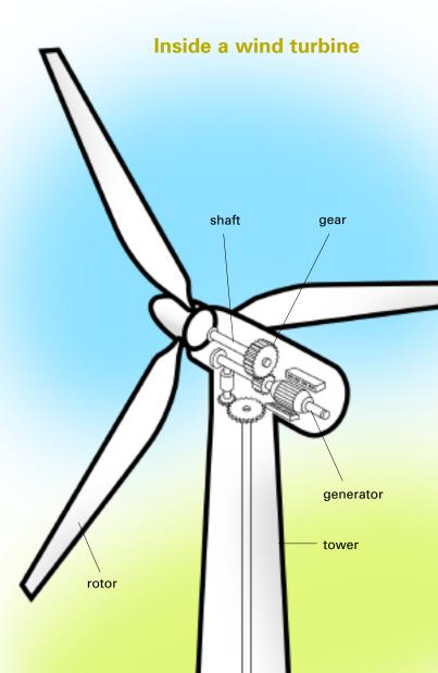
To produce power, you need a wind speed of at least four metres per second (around 14KPH). Wind speed increases as you go higher above ground level, so wind turbines are usually mounted on tall towers. Wind speed also increases if there are no hills or buildings to slow it down. It is normally windier at sea than on land.
