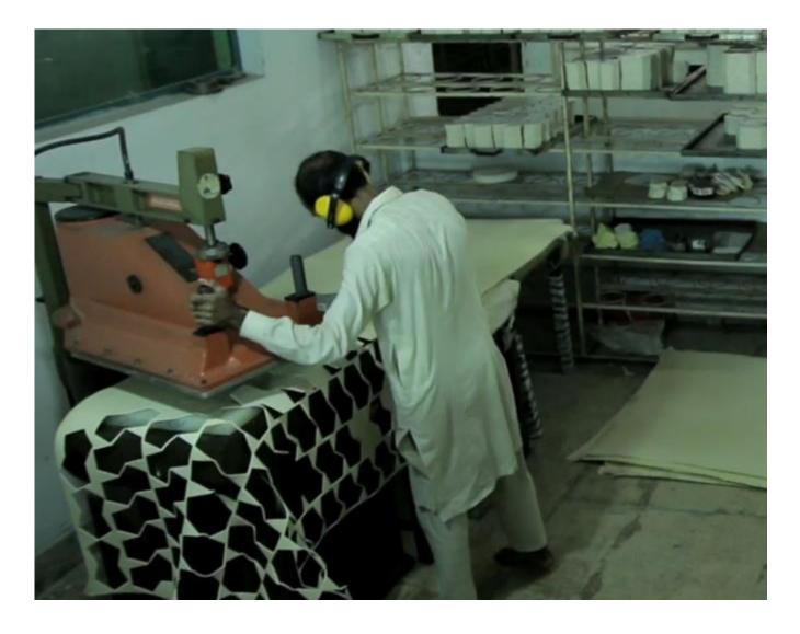
The pieces are cut using a large, loud machine – note the ear protectors!
