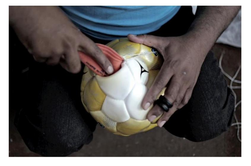
Only at the end is the ball turned around the right way and an air-bladder is inserted so that the ball can be inflated.
